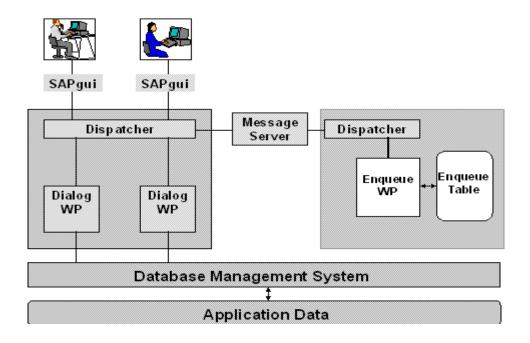
The enquire function module sets an SAP lock by writing entries in the central lock table. If the lock cannot be set because the application object (or a part of it) is already locked, this is reflected in the return code sy-subrc. The following diagram shows the components of the R/3 System that are involved in setting a lock.
