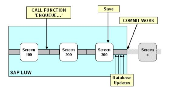
These function modules are executed in a special enquire work process. Within an R/3 System, enquire work processes run on a single application server. This server maintains a central lock table for the entire R/3 System in its shared memory.
