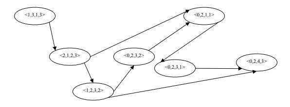
Once the learning is over each user has a user access graph where each node in the graph represents the fingerprint of the transaction. Based on this information we proceed to detection phase.
